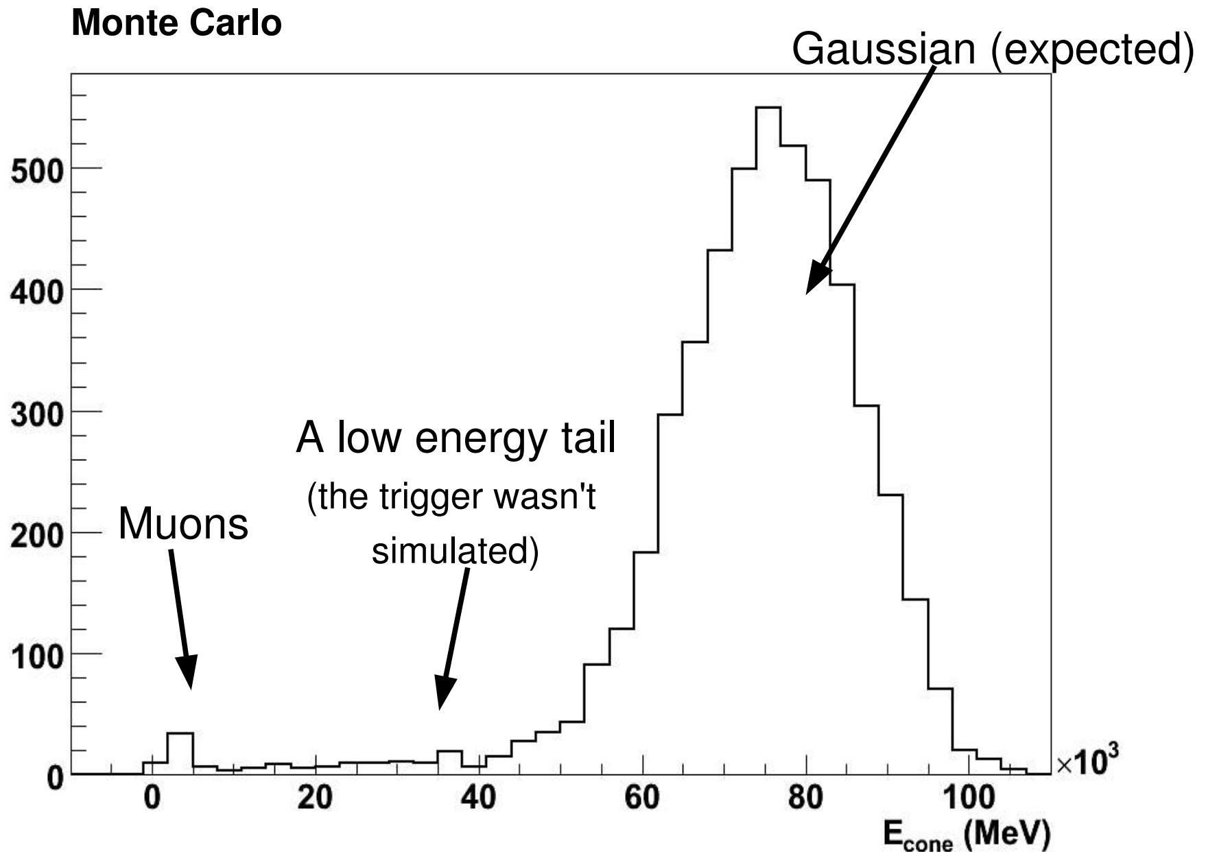
Energy cone for  $E_{\text{beam}} = 9 \text{ GeV}$ ,  $\eta = 0.35$ , opening angle  $11^\circ$
