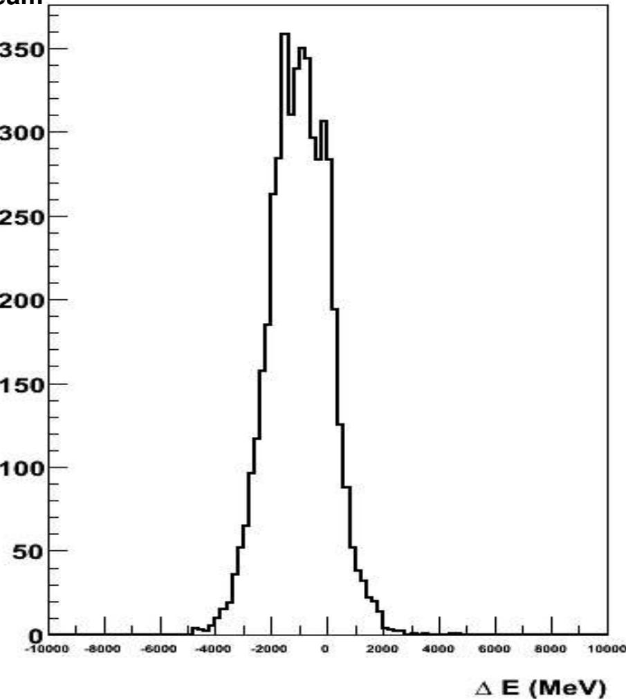
$E_{\text{weight}} - E_{\text{total CalibHit}}, E_{\text{beam}} = 100 \text{ GeV.}$
