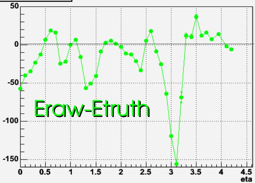
Similar behaviour as jet samples, but more clear effect of crack can be observed.
