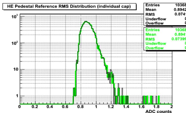
Pedestal value ~ 3 ADC/TS and event to event RMS of pedestal ~ 0.7 ADC/TS
