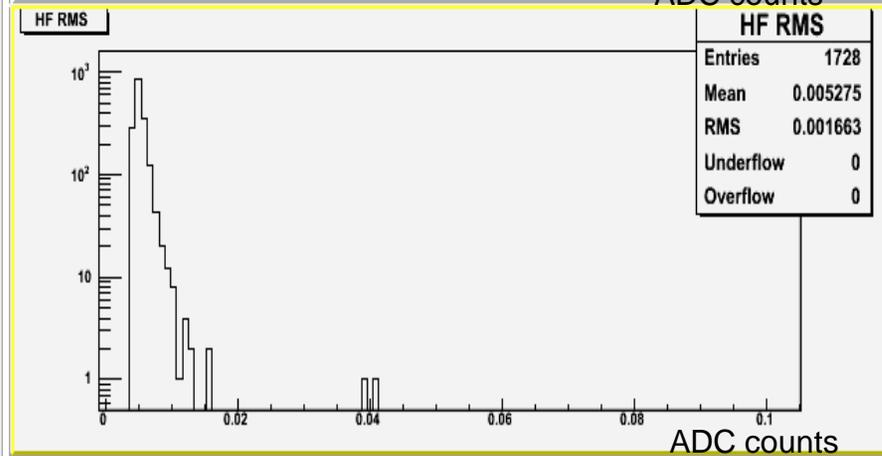
Average run-to-run RMS per subsystem  $\sim 0.004$  ADC/TS
