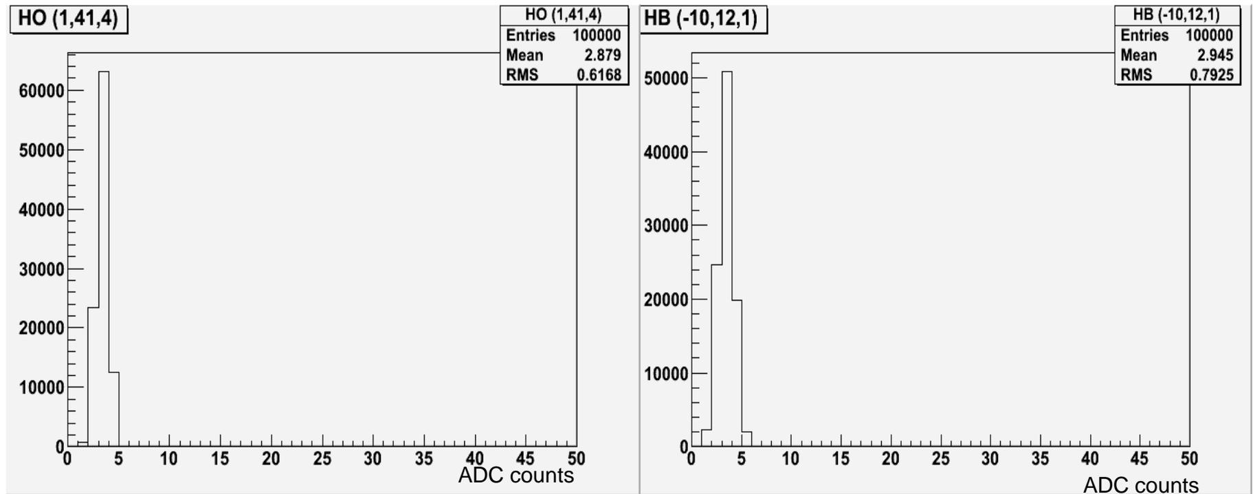
A typical pedestal signal in ADC counts
