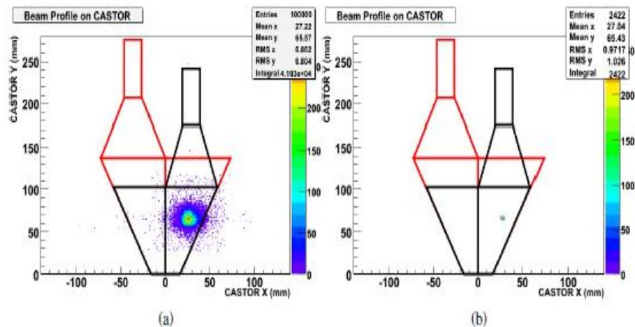
1. Beam Profiles of 100 GeV electrons impinging on center of the Saleve side.(Run 47601)
