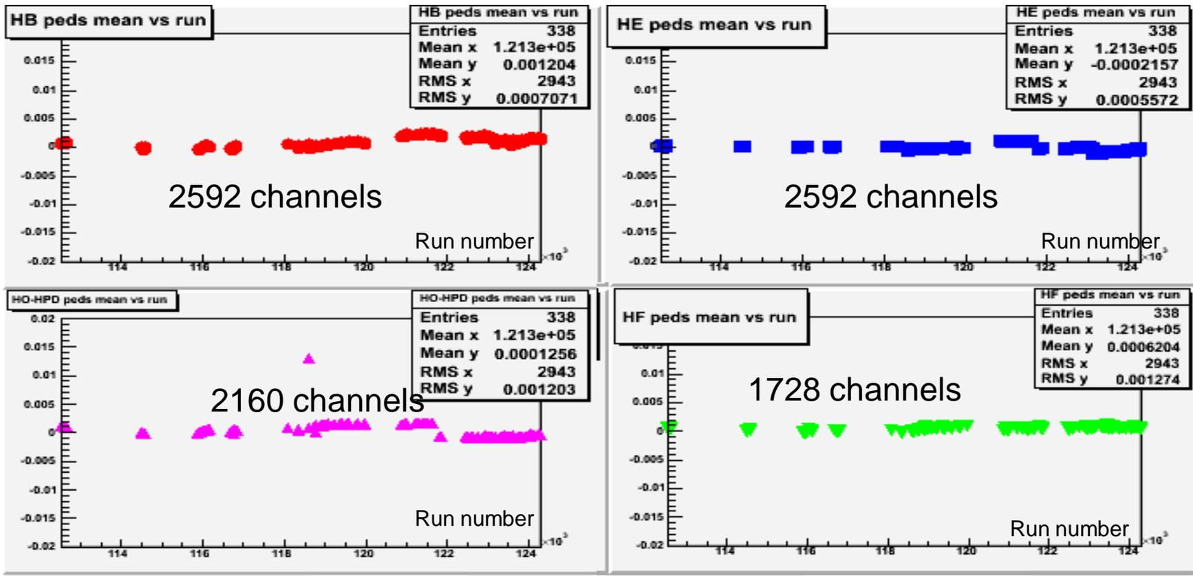
Each point shows the difference between pedestal mean value averaged over all channels for a given run and the value in reference run
