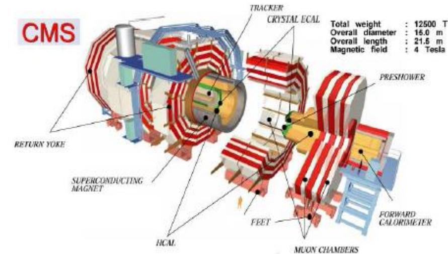
➤ CMS is multi-purpose detector designed to measure both single particles (electrons, photons, muons) and particle jets (e.g. hadronic jets or tau-jets)
