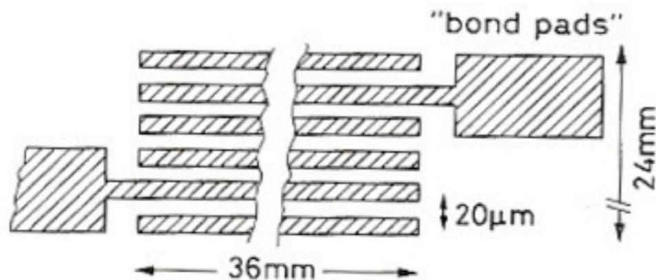
**Fig. 10.16.** Layout of a micro-strip detector and readout strips (from *Hyams et al.* [10.14])
