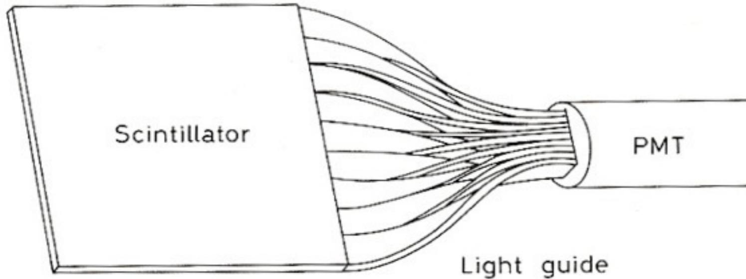
**Fig. 9.7.** The *twisted* light guide. Many strips of light guide material are glued on to the edge of the scintillator and then twisted  $90^\circ$  so as to fit onto the PM face
