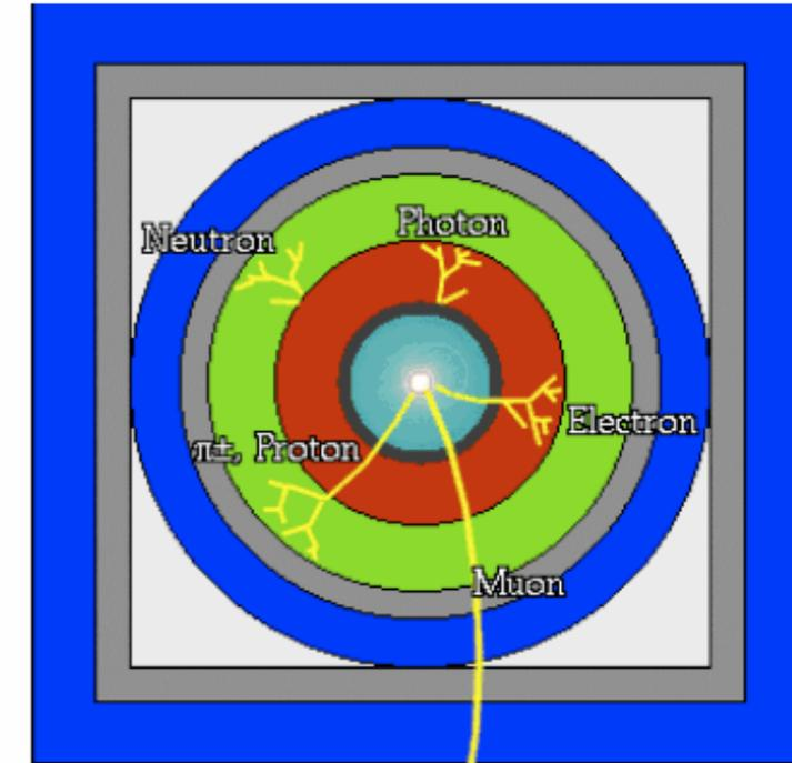
**Tracker:** Momentum of charged particles via precise measurement of deflection in magnetic field
