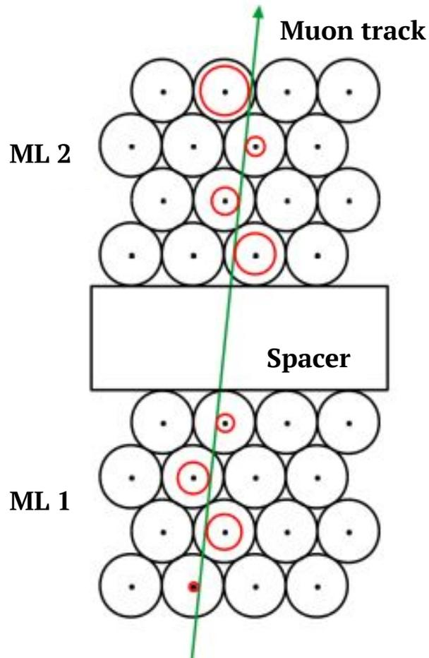
sMDT (**s**mall **M**uon **D**rift **T**ubes) chambers are used as precision tracking detectors
