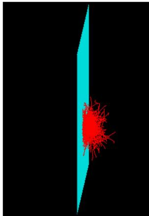
GEANT4 simulation. 70keV electrons couldn't go through the Kapton window of our GEM chamber. Red lines are 70 keV electrons
