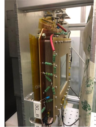
Fig 4. Picture of GEM with HV divider
