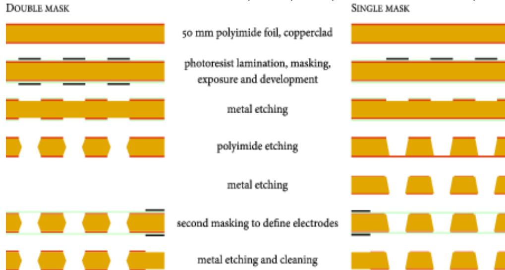
Fig 1. Double Mask and Single Mask
