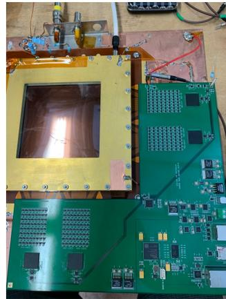
Fig 3. Picture of Developing 2D DAQ and GEM
