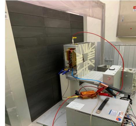
Thermal neutron field at the Korea Research Institute of Standards and Science (KRIS). The field was produced with high rate  $^{241}\text{Am-Be}$  Source and a high purity graphite blocks. Ref [3]
