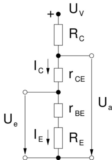
$$dI_E = \frac{dU_e}{r_{BE} + R_E} \approx \frac{dU_e}{R_E} \quad (r_{BE} \ll R_E)$$
