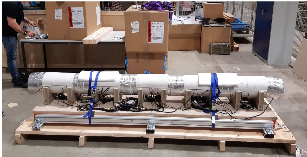
Heavy lifting: 500 kg of electrically-heated prototype
