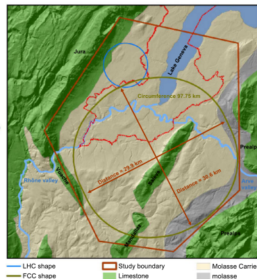
Fig. 2. Left: 3D, not-to-scale schematic of the underground structures. Right: study boundary (red polygon), showing the main topographical and geological structures, LHC (blue line) and FCC tunnel trace (olive green line).
