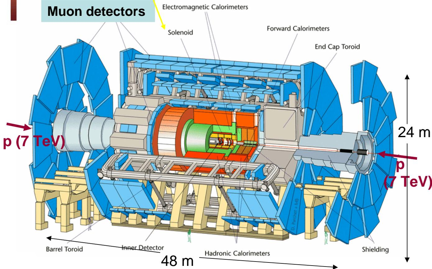
The **ATLAS muon spectrometer**:
