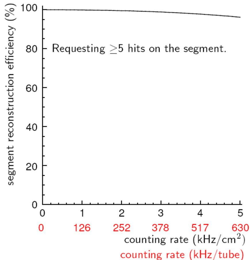
Simulation: 8 layer chamber with 15 mm diameter and 80 cm long tubes (Oliver Kortner)
