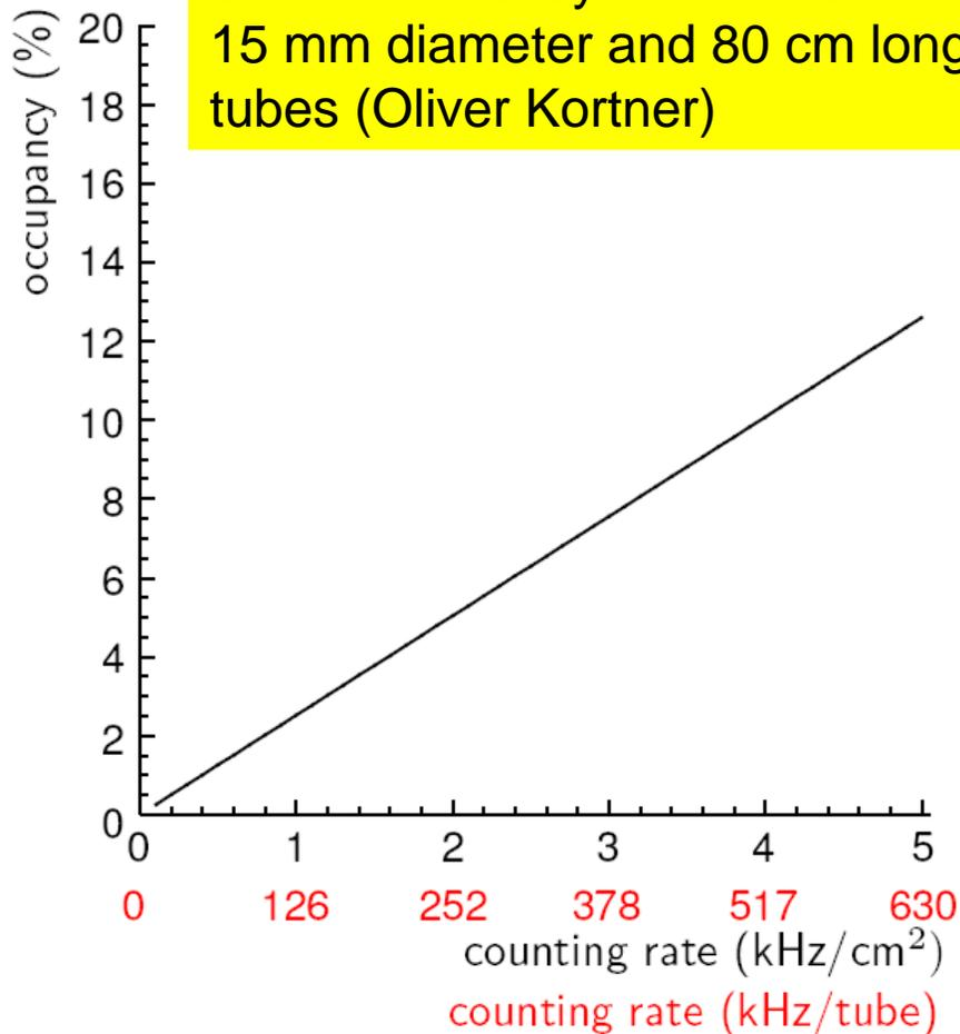
Number of muon hits in an 8-layer chamber
