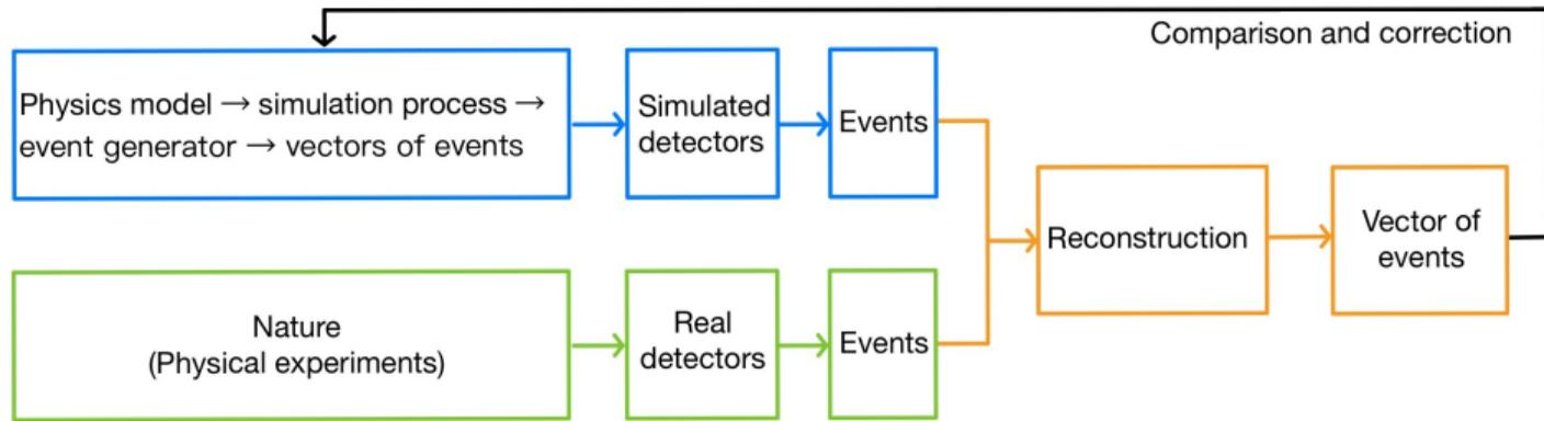
**Figure 6** Event generation, detection and reconstruction.
