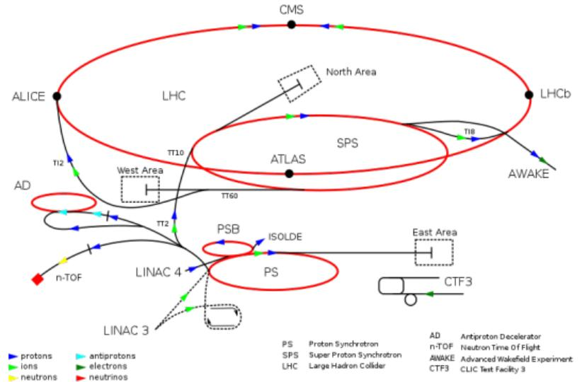
Figure 4 CERN accelerator complex.
