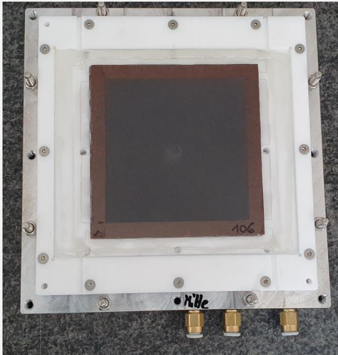
The second bonding stage prepared with the glue.
