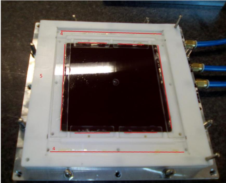
The first bonding stage. The red lines mark the position of the glue traces.
