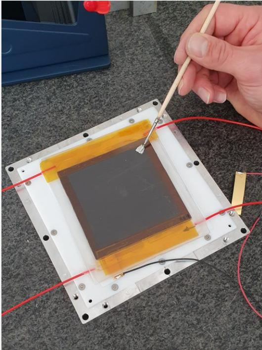
Application of the conductive silver adhesive to strengthen the contact of the electrode.
