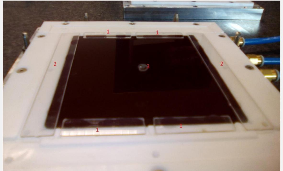
Four small spacers (1) leave space for six gas channels, two long spacers (2) seal the side and a c-shaped spacer (3) in the middle of the plate.
