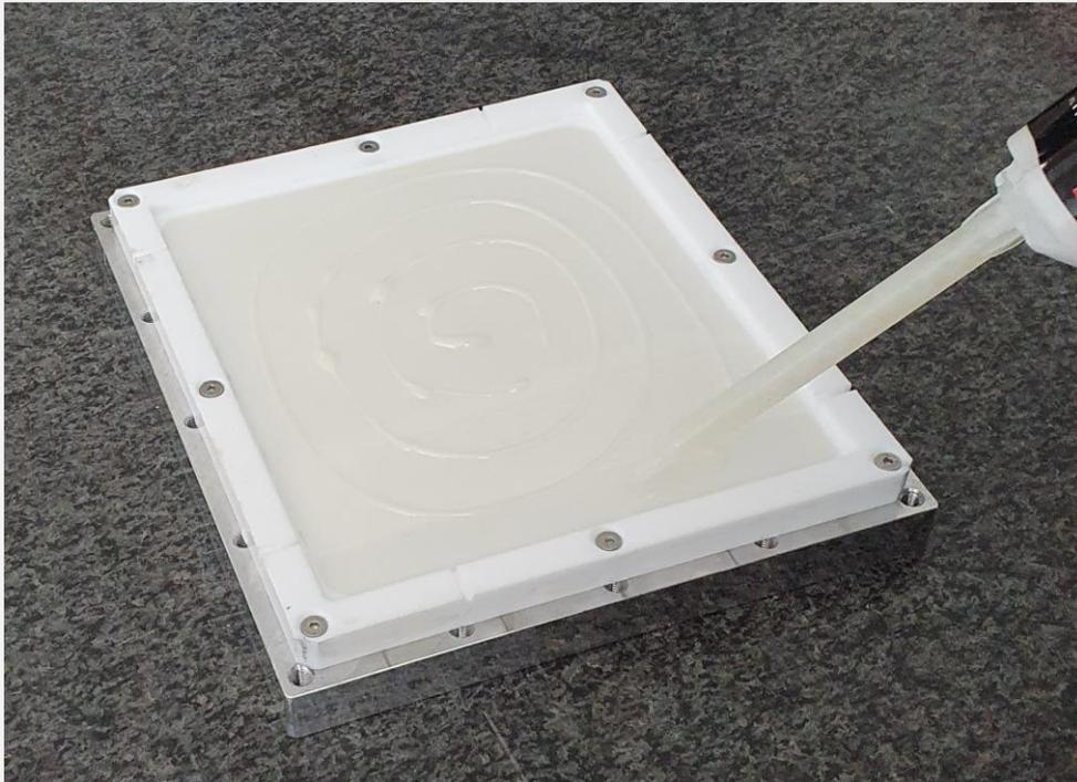
The gluing of the lower mylar foil. The glue needs to get spread out evenly.
