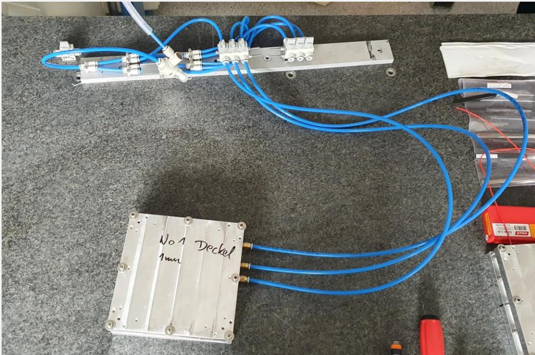
The first bonding stage connected to the vacuum pipe system.
