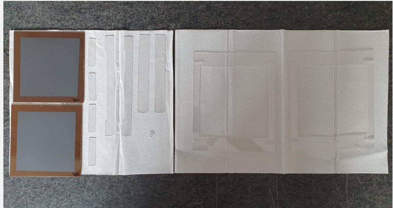
Plates and polycarbonate parts for the three bonding stages. From left to right: Graphite coated Pertinax plates, spacer and parts for the gas channels (nine), two outer frames.
