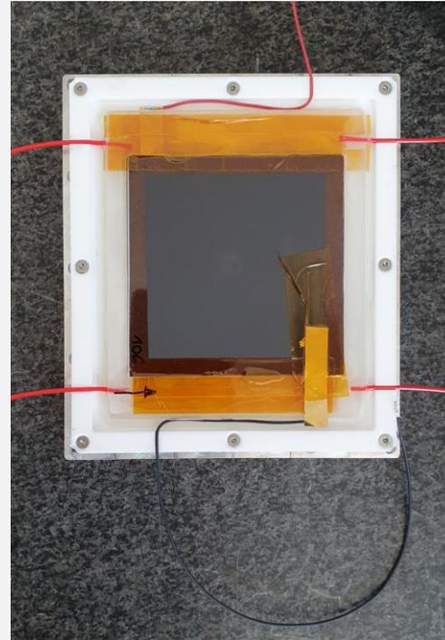
The electrodes fixed to the plates with Kapton tape
