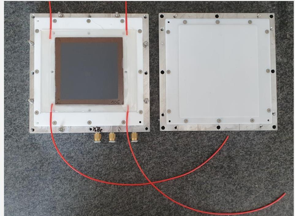
The second bonding stage with all parts in place.
