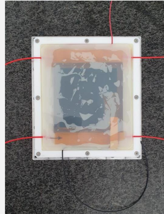
The third bonding stage before the the drying process.
