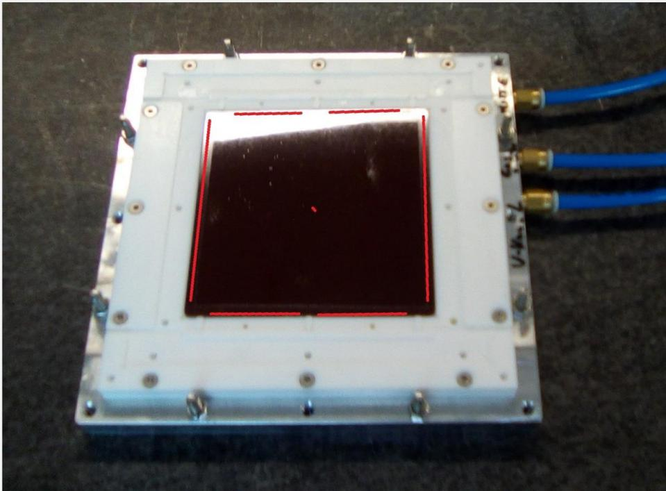
The first bonding stage. The red lines mark the position of the glue traces.
