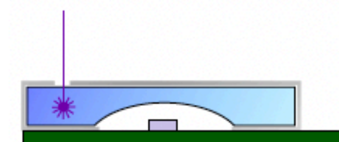
Inject pulsed laser beam into scintillator tile
