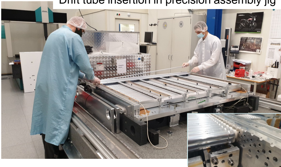
Drift tube insertion in precision assembly jig
