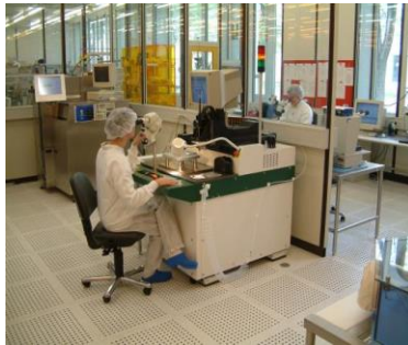
Wire bonding, hybrid assembly
