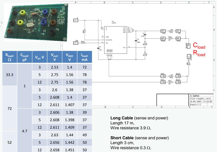
By choosing a capacitor (CVS) of 1 µF between the regulator output pins and the sense return line, the oscillation disappeared completely.
