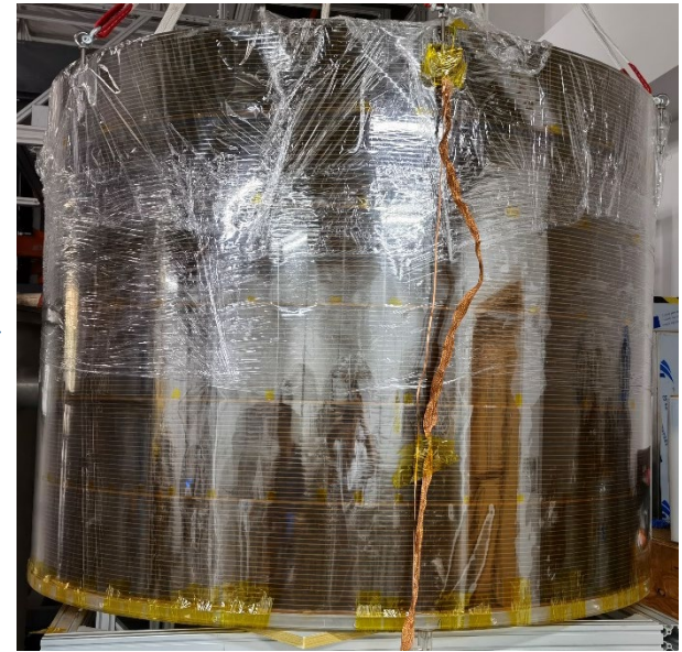
First Phase TPC (52 MMs)
