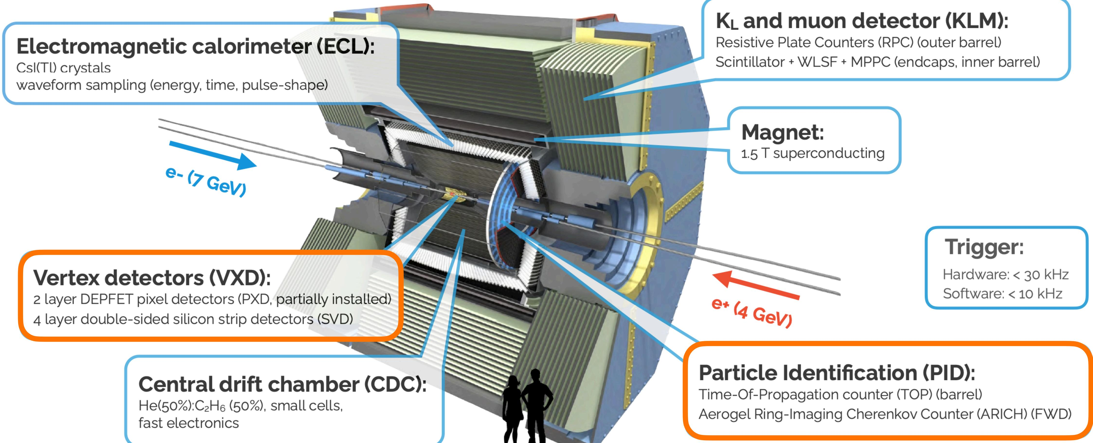
DEPFET: depleted p-channel field-effect transistor
