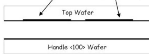
b) wafer bonding and grinding/polishing of top wafer
