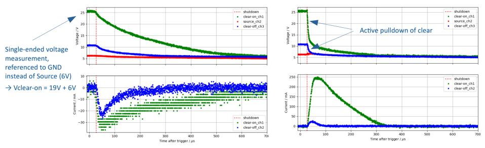
All measurements done with Hybrid5 PCB without ASICS&matrix, but all SMD components  $\rightarrow$  Active pulldown significantly decreases shutdown time
