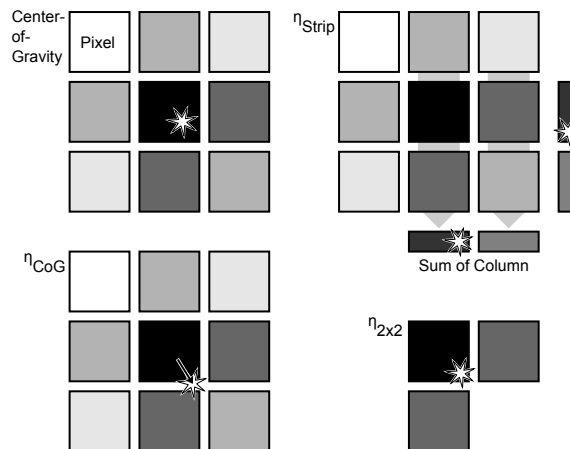
Figure 5.11: Schematic representation of four PFA. The CoG algorithms systematic bias is corrected in the \eta_{CoG} as indicated with the gray arrow. \eta_{Strip} combines pixel columns (rows) considering only the two highest strips whereas \eta_{2x2} considers the two highest pixel signals in the seed row (column) to estimate the point of passage.
