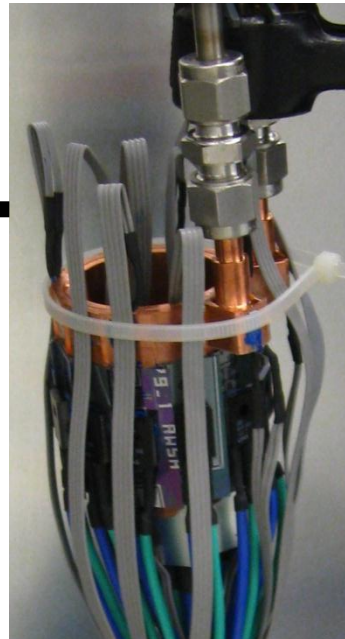
Endflange prototype with load resistors and Pt1000s
