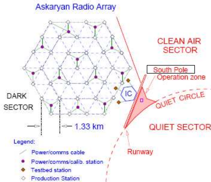
Figure 2: Planned layout of the 37 ARA stations with respect to the South Pole Station and associated sectors.
