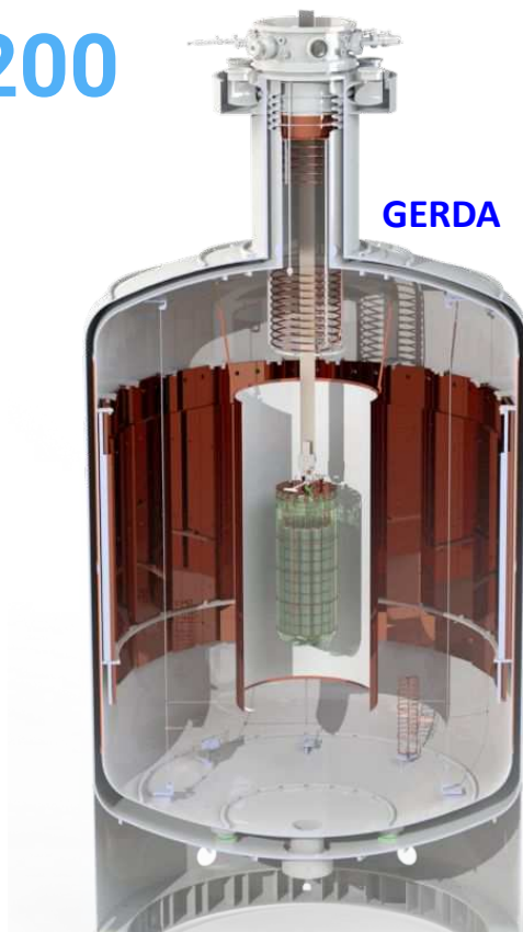
Liquid argon tank ( 64\text{m}^3 ) Pure water tank ( 600\text{m}^3 )
