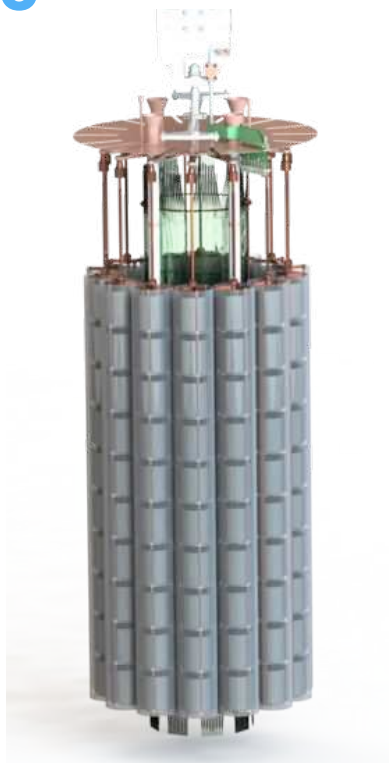
Detector arrays with copper holding structure
