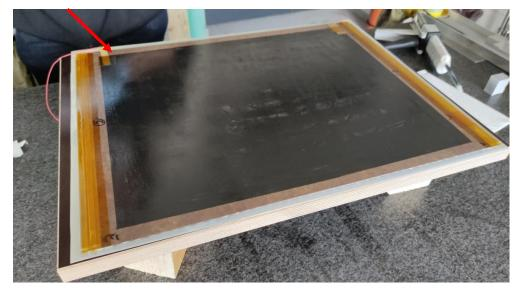
**Insulating:** The PET foil with pre-applied Ethylen-Vinylacetat (EVA) is placed on outside of electrodes and heated up with heating mats
