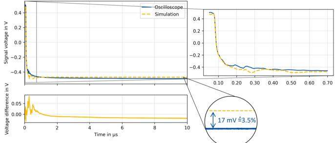
• Amplitude mismatch in measurement and simulation
