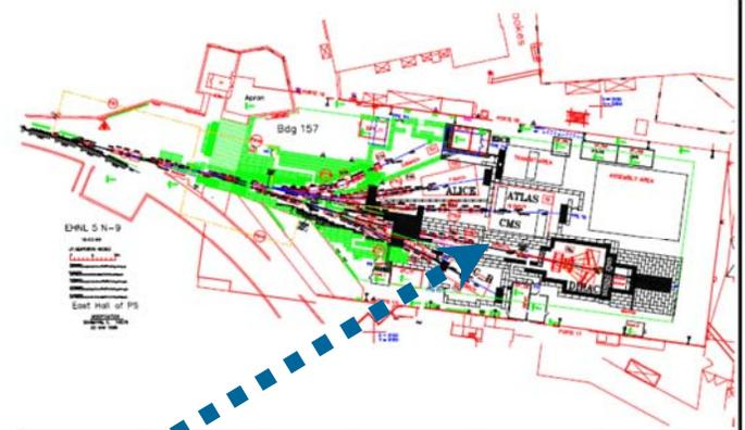
Figure: Beam lines in the PS East Hall. T7 and T8 are near the bottom. The maximum length is below 100 m.
