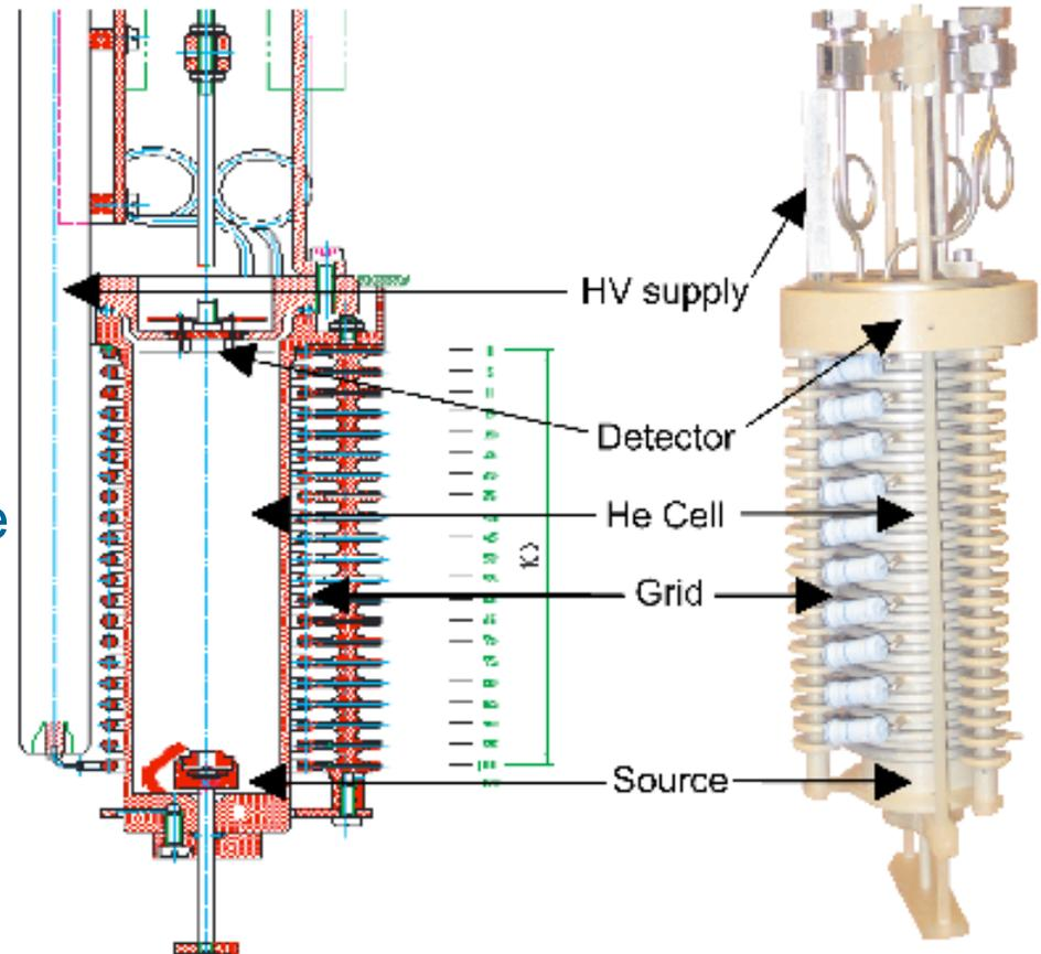
The Frictional Cooling Demonstration Experiment is searching for a new method of efficiently reducing the beam emittance
