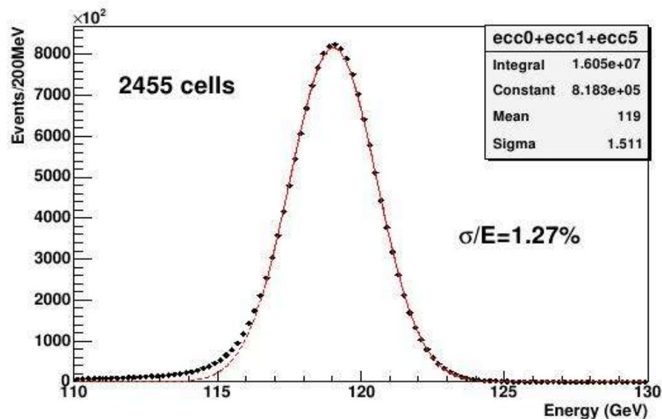
Energy resolution at 120 GeV for 3 beam-tested EMEC modules (2455 cells  $\sim 3 \text{ m}^2$  of detector).
